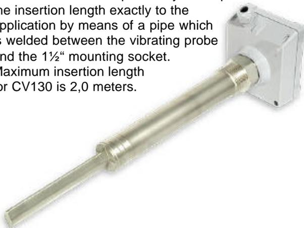
The CV130 is suitable for top mounting. Side mounting is possible for insertion lengths shorter than 1 meter and if the extension pipe is adequately supported. Connection to the container is made via thread 1 ½" DIN (equals BSPT) or NPT.
